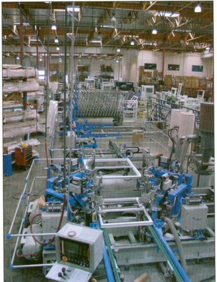
Vinyl fabricating machines allow the manufacturer to process numerous different sash and profiles on the same line without lost time for set-up.
