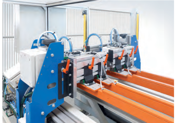
Linear Motion pusher system with optional four gripper configuration
