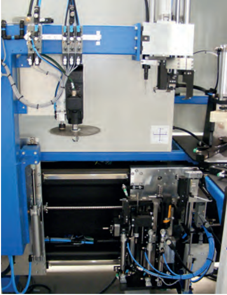
Four axes control (interior view)
